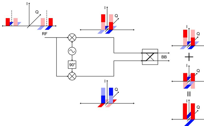
Figure 5.1: Working principles of a sideband rejection IQ mixer
