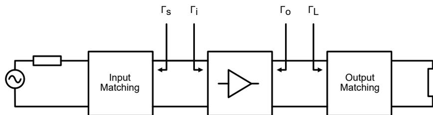
Figure 4.1: Matching networks at the input and output of an amplifier.
