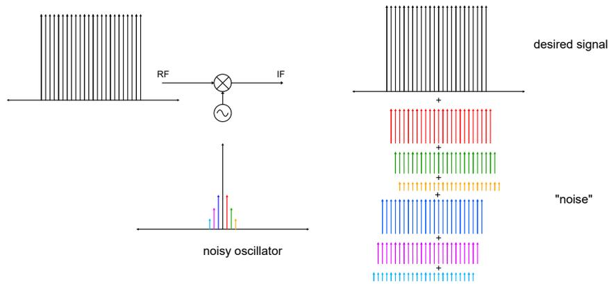
Figure 6.1: Effect of LO phase noise on OFDM signals
